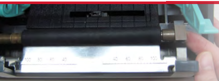
Platen Roller Structure — easy access for quick change
